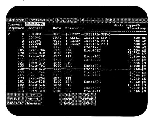
Figure 6-3 Disassembly menu (68010 Control Flow format)
