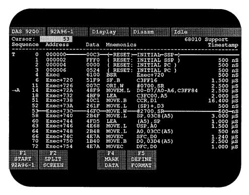
Figure 6-2 Disassembly menu (68010 Software format)
