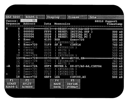
Figure 6-1 Disassembly menu (68010 Hardware format)
